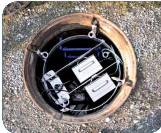
Pic: Two emovable boxes (IP 68) for battery pack and data logger/modem housing - easy to access, easy to exchange, easy to store. All tight and water-proof.
