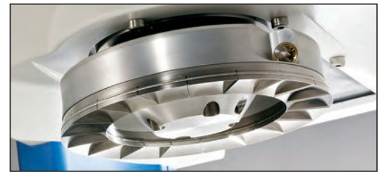
Close-up View of Vane Lid used for Flow Function Test.
